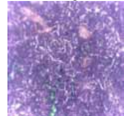
Filter Failure - Fibres & Contamination
