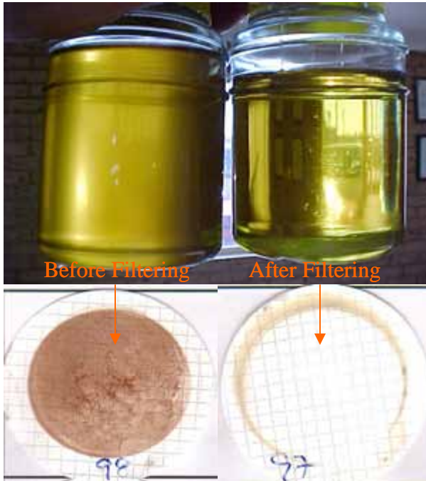
Above are 0.8 micron filter patches done before and after running the samples through the FF 3000
